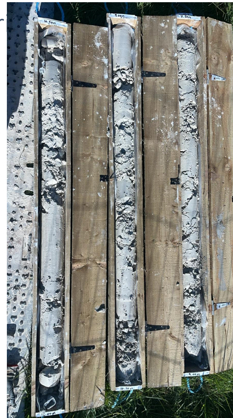
Geological cores retrieved of the underlying Chalk
